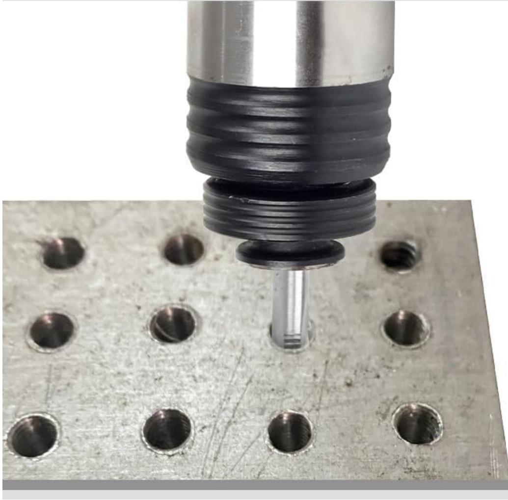
Figure 6: The tapping machine actively engaged in a tapping operation, illustrating its strong force and good quality performance on a metal workpiece. This image emphasizes the tool's capability in creating precise threads.
