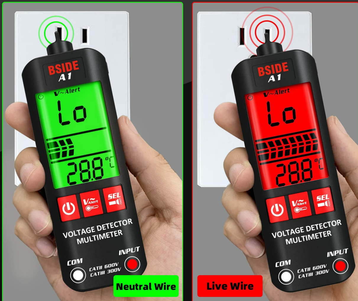
Figure 6.3: Distinguishing between neutral and live wires using the multimeter's detection feature.
