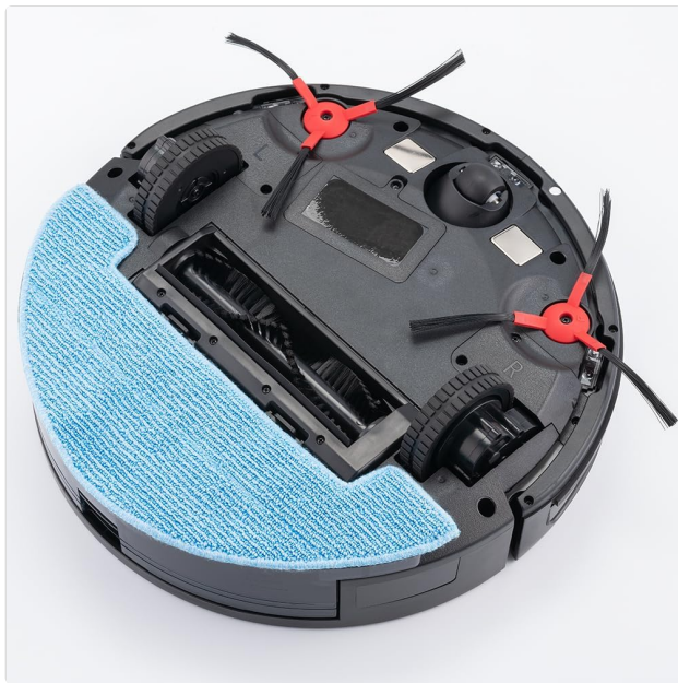
Figure 2: Bottom View with Mop Pad. This image displays the underside of the robot vacuum, featuring the main brush, side brushes, wheels, and a blue microfiber mop pad attached to the water tank. This configuration is used for wet mopping.
