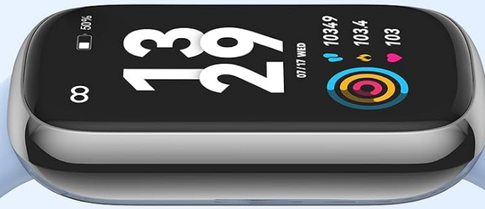
Figure 3: The 1.47" HD color touchscreen displaying various functions and customizable watch faces.
