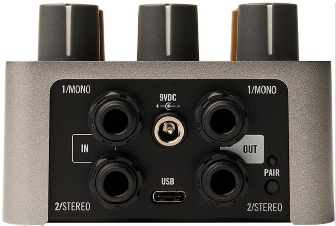
Figure 4: Rear panel of the Universal Audio OX Stomp pedal, showing input/output jacks, power, and USB port.
