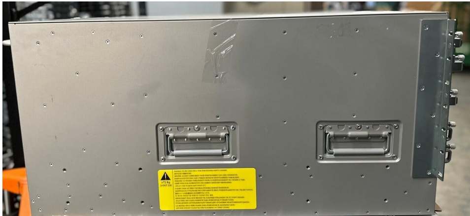
Figure 4: Side view of the chassis. This image highlights the side handles for maneuvering and a warning label indicating the substantial weight of the empty chassis (372 kg / 820 lbs), emphasizing the need for proper lifting equipment.
