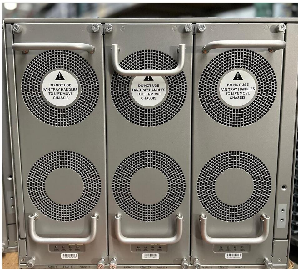
Figure 3: Rear view of the chassis with fan trays. Each fan tray has a clear warning label stating, "DO NOT USE FAN TRAY HANDLES TO LIFT/MOVE CHASSIS," emphasizing proper handling procedures.
