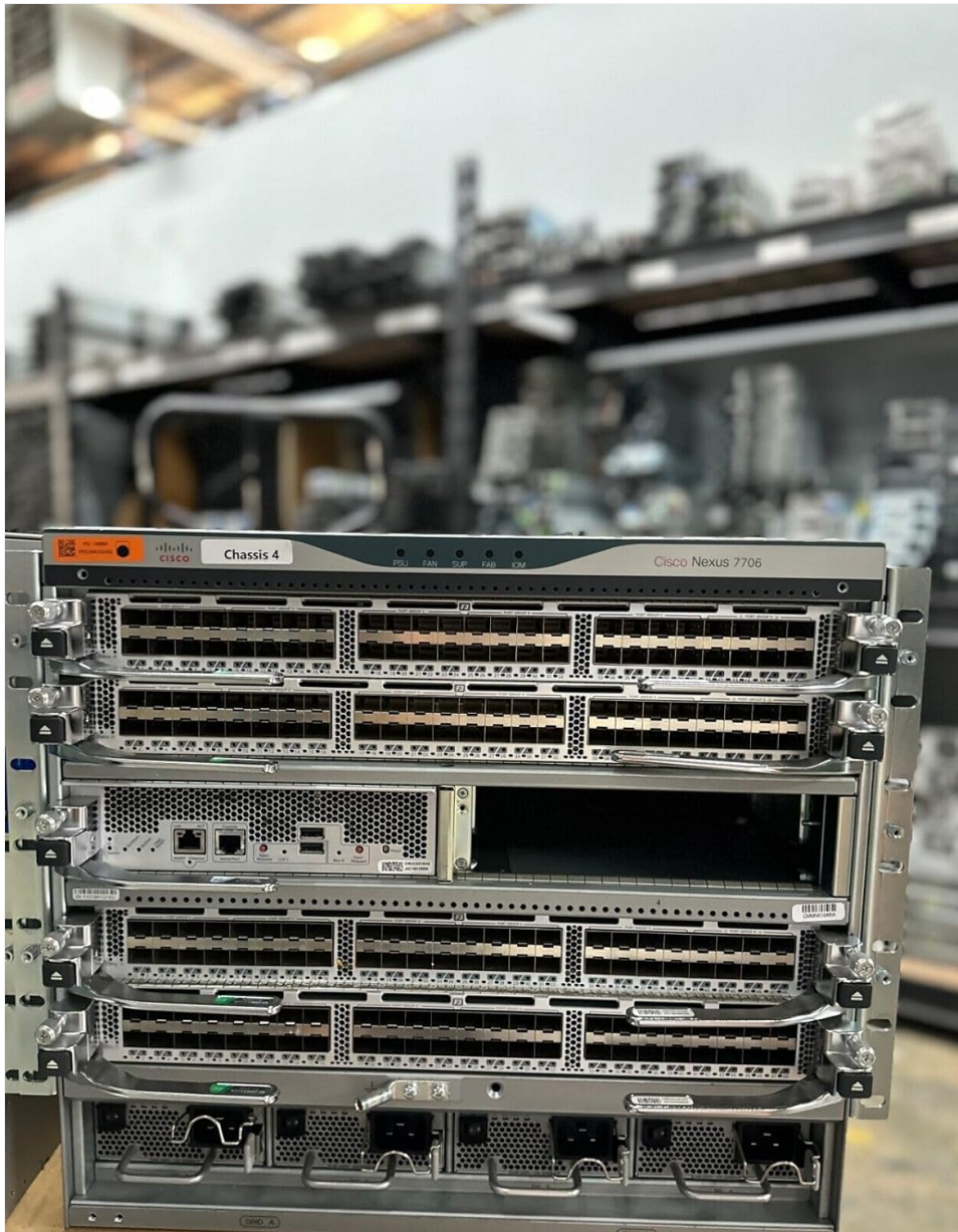
Figure 1: Front view of the Cisco Nexus 7706 chassis. This image displays the modular design, showing slots for supervisor engines, fabric modules, and line cards, along with the Cisco Nexus 7706 branding.
