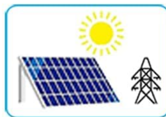
Solar Priority (Utility as backup power)
