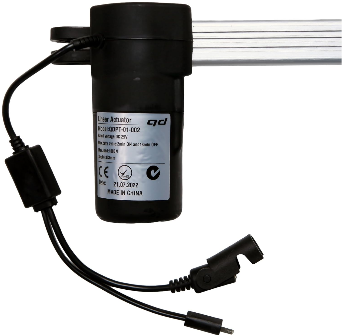
Image: Close-up of the product label, detailing the model number QDPT-01-002, rated voltage DC 29V, max duty cycle 2min ON and 18min OFF, max load 1000N, and stroke 333mm.
