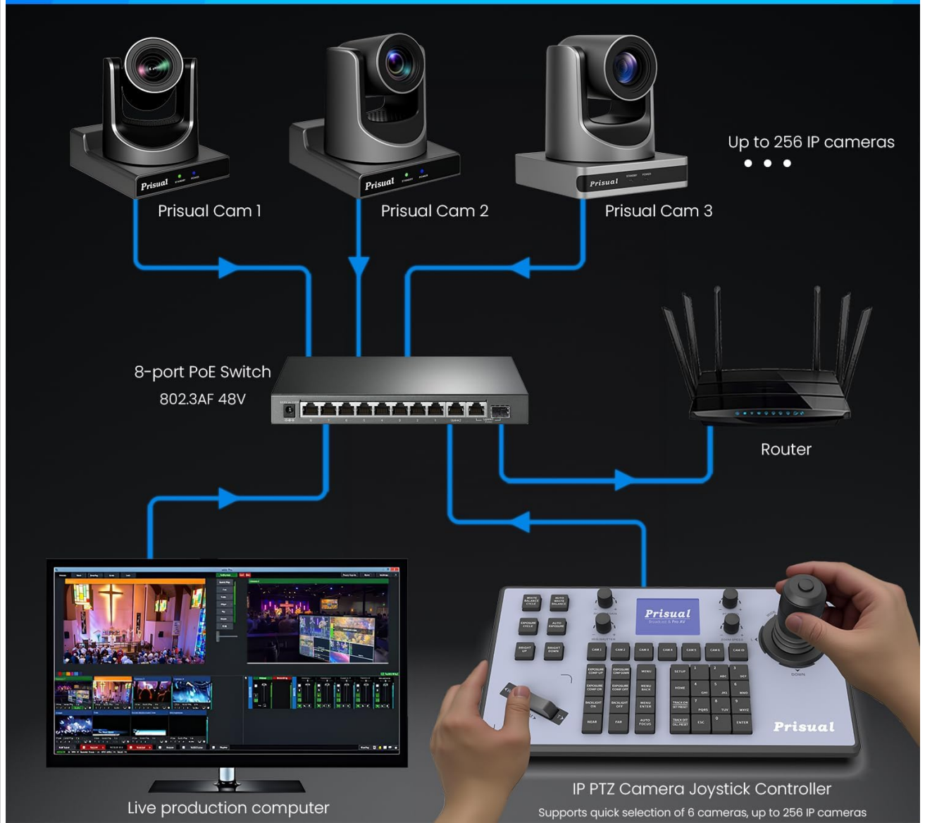
Figure 3.3: Example setup demonstrating how the Prisual TEM-JOY1 controller connects to multiple PTZ cameras and a live production system via a PoE switch.
