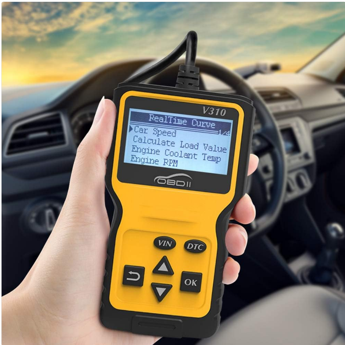
Figure 5: The V310 scanner displaying real-time data such as Car Speed, Calculated Load Value, Engine Coolant Temp, and Engine RPM.
