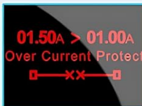
Overcurrent automatic power off alarm interface
