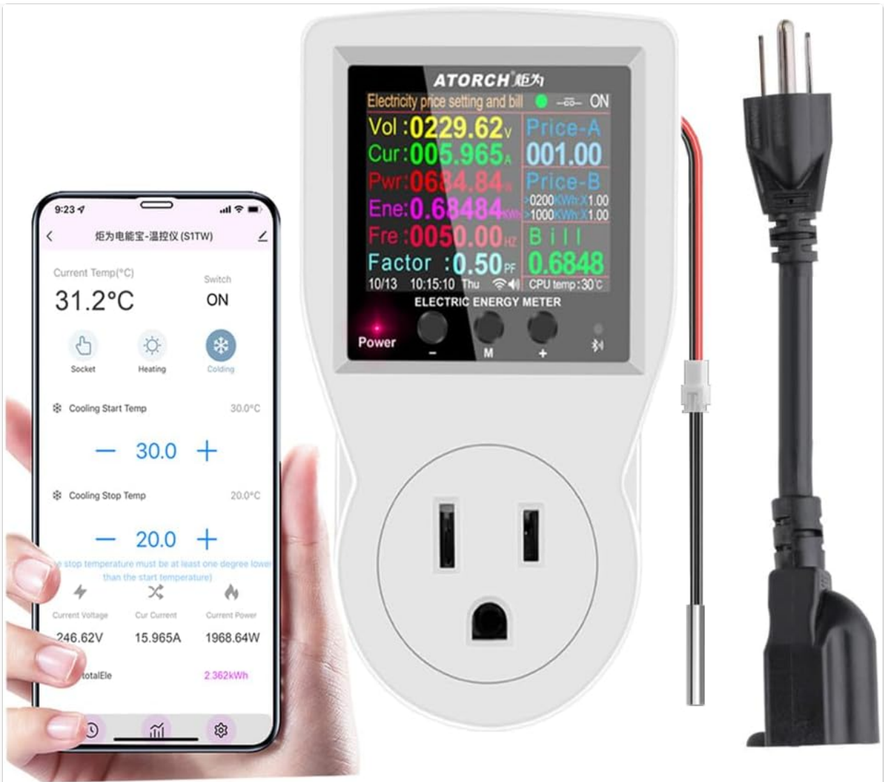
Figure 1.1: AVHzY AC WiFi Watt Meter S1TW with its external temperature probe and power cable.
