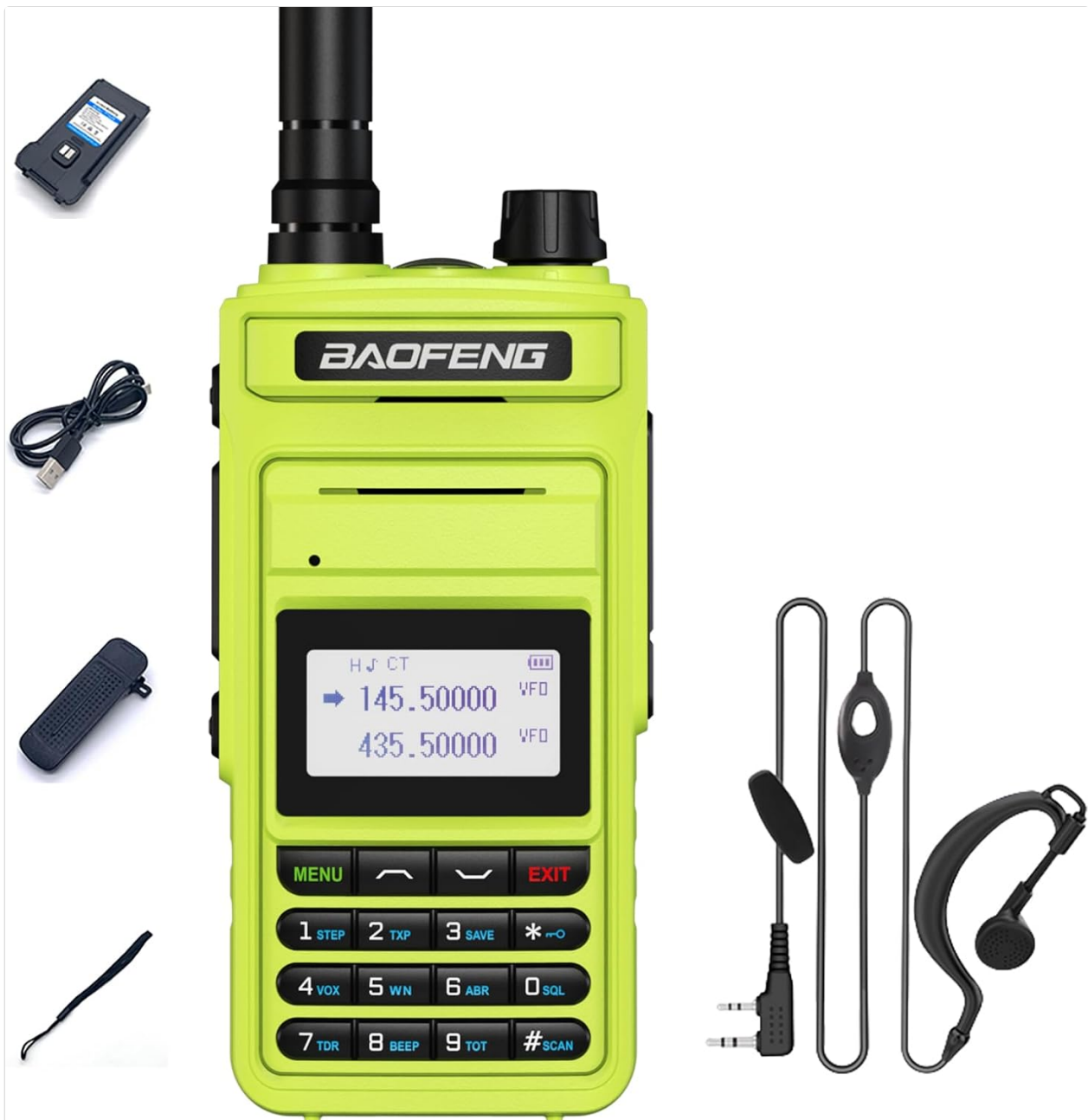
Image 2.1: The BAOFENG P15UV radio shown with its complete set of accessories, including the antenna, battery, USB-C cable, belt clip, hand strap, and headset.
