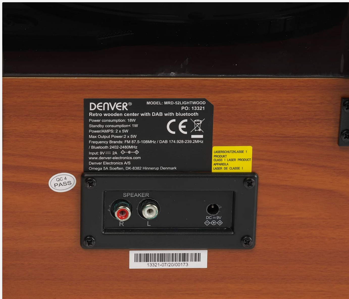
Figure 5: Detailed view of the speaker terminals (R and L) and the DC power input on the rear of the unit.
