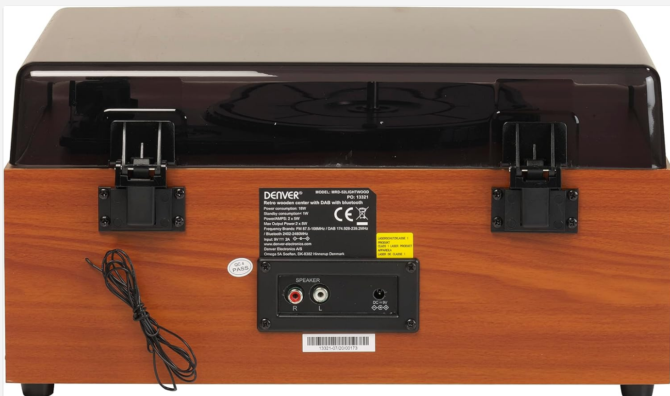
Figure 3: Rear view of the music system, showing the speaker output terminals and power input.
