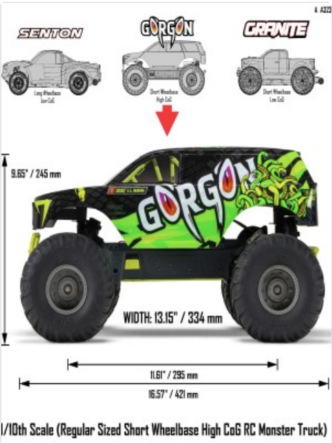
Image: Side profile of the ARRMA Gorgon RC Truck, illustrating its physical dimensions.
