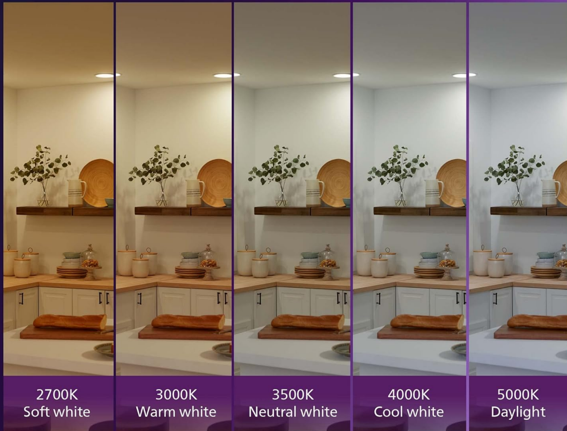
Image: A visual representation comparing various shades of white light, from 2700K Soft White to 5000K Daylight, illustrating color temperature differences.
