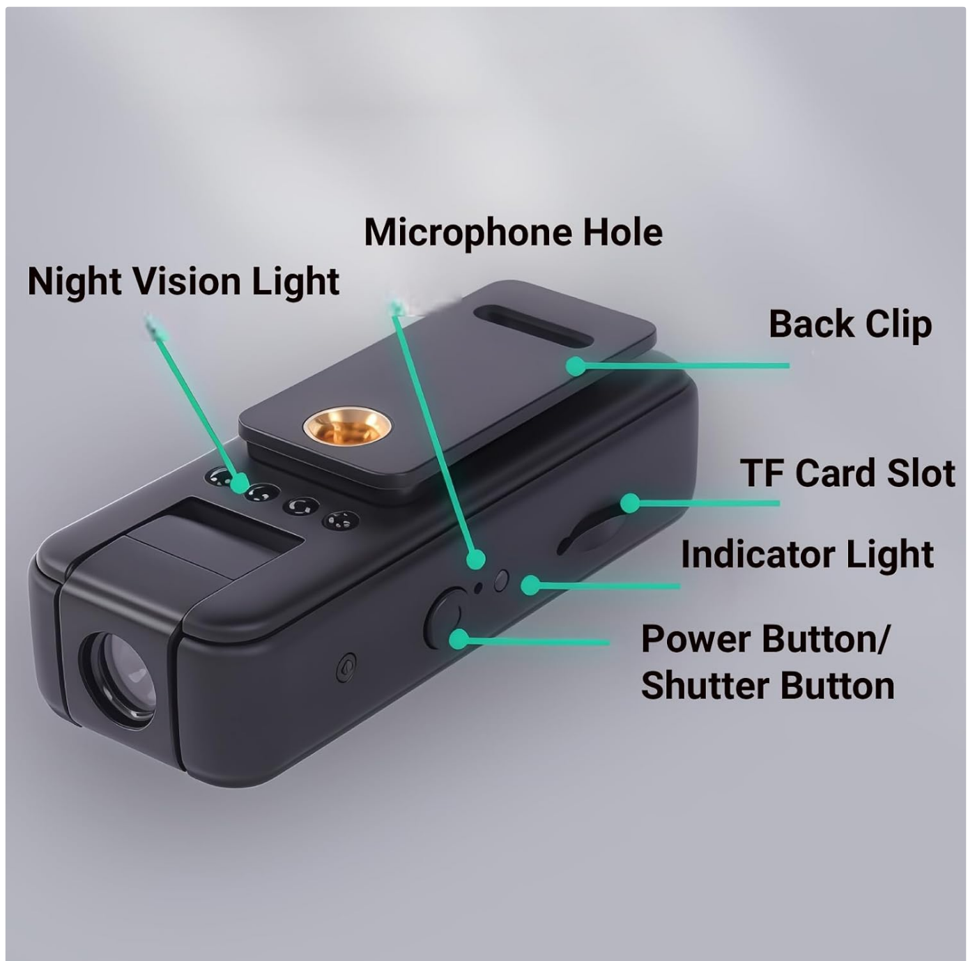
Image: Top and back view of the camera with key components labeled, including night vision light, microphone hole, back clip, TF card slot, indicator light, and power/shutter button.
