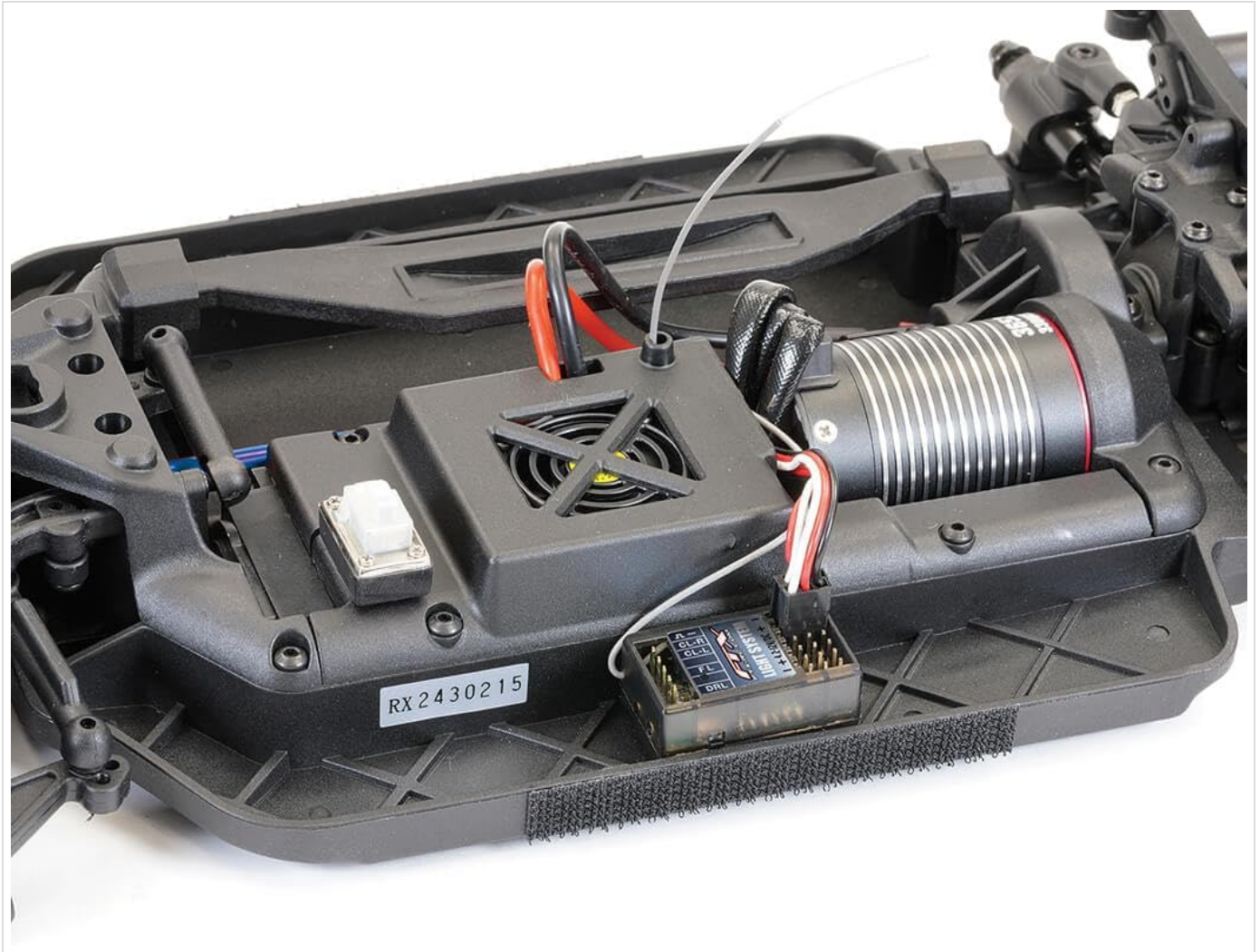
Image: A detailed view of the FTX Stinger's brushless motor and Hobbywing 60A ESC, showing the cooling fan and wiring.
