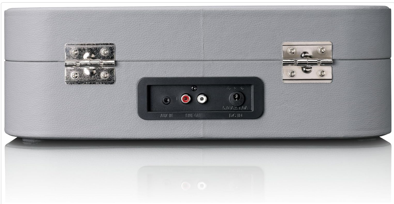
Figure 4.2: Rear view of the Lenco TT-116 Turntable, highlighting the AUX In, Line Out (RCA), and DC In power ports.
