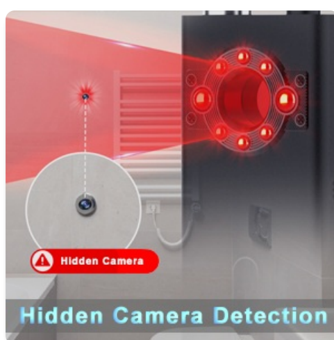
Figure 6: Infrared mode helps locate hidden camera lenses.
