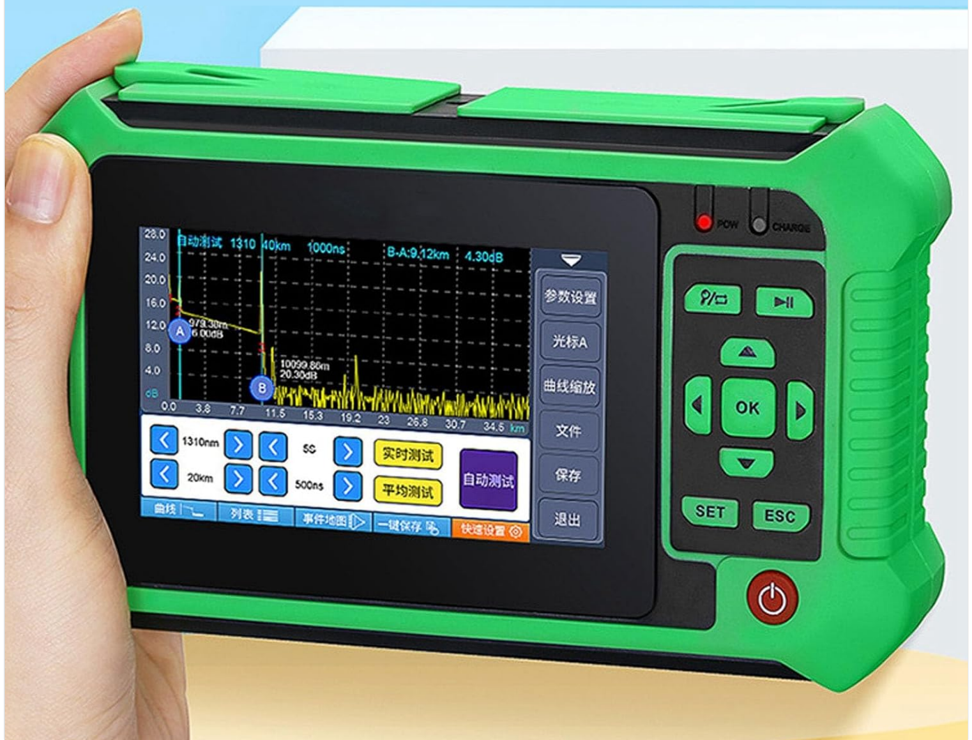
Figure 4: The automatic test analysis screen displaying an OTDR trace with event markers and measurement data.
