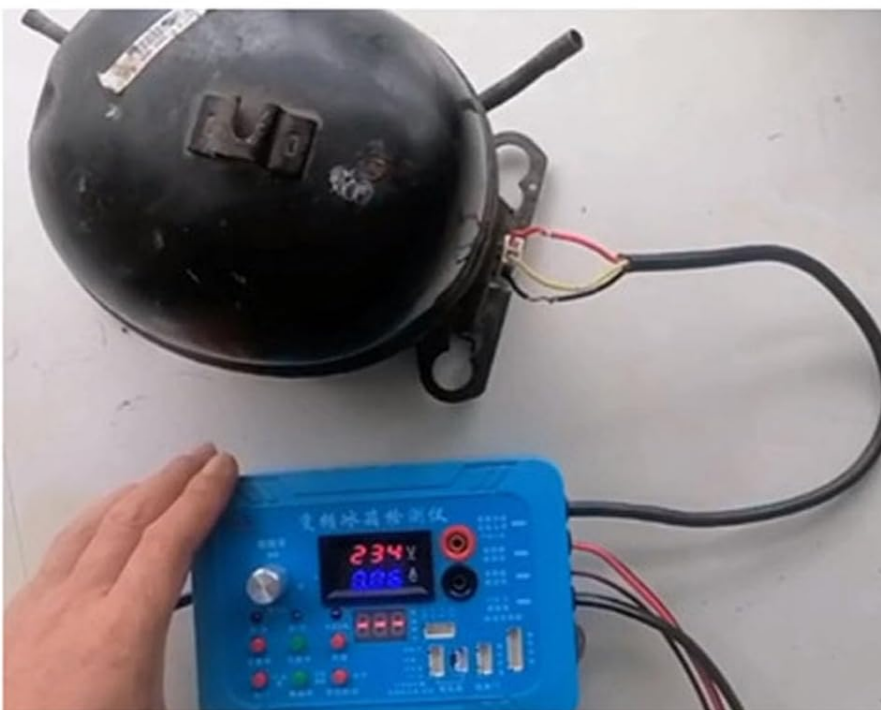
Figure 6: The testing instrument connected to a refrigerator compressor, demonstrating the setup for diagnosing or attempting to repair a jammed compressor.
