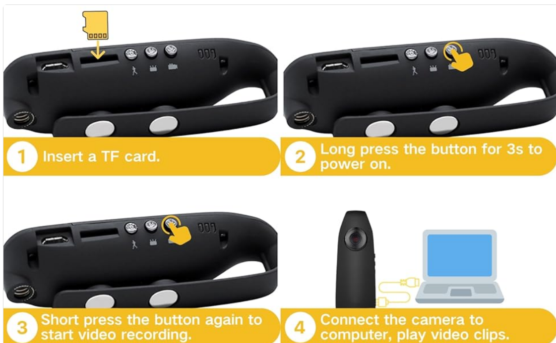
Image 3.1: Step 1 illustrates inserting the TF card into the camera.
