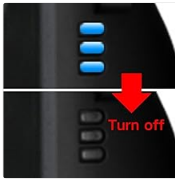
Image 4.1: Indicator lights showing power on (blue lights) and power off (lights off).
