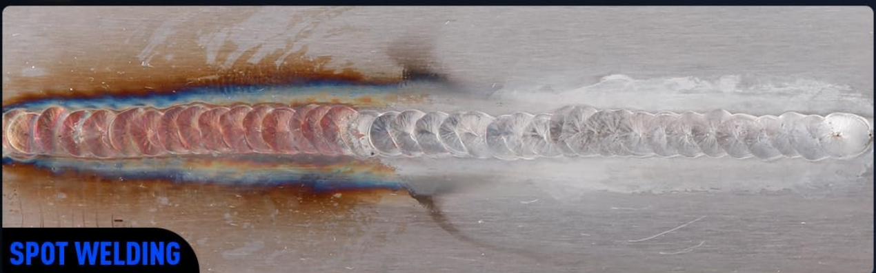
Figure 5.2: Visual examples of weld beads produced using TIG, Pulse TIG, and Spot Welding functions.
