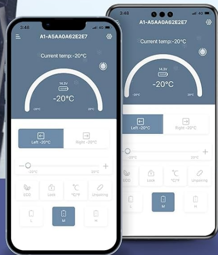
Image 6.1: The control panel displays current temperature, battery voltage, and active mode, with buttons for power, settings, and temperature adjustment.
