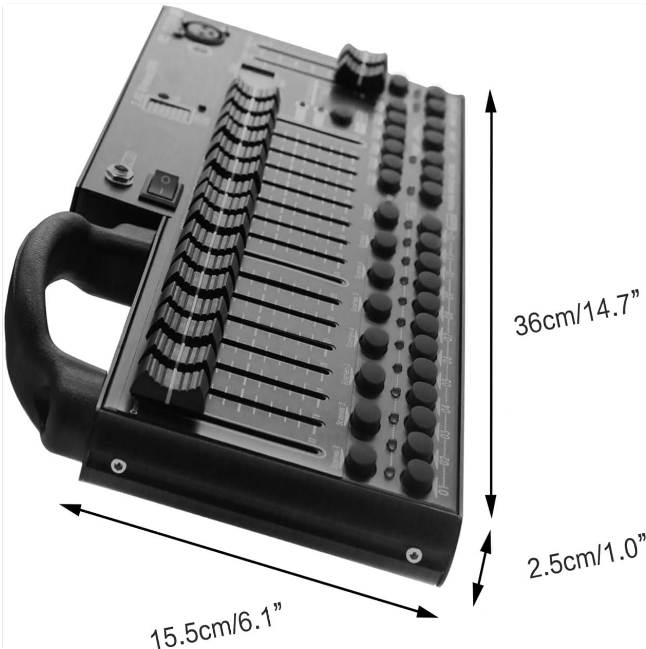
Figure 3.2: Example of the DMX 384 controller used with different types of DMX lighting fixtures.
