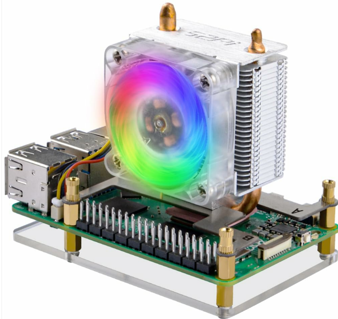
Image 1.1: GeekPi ICE Tower Cooler mounted on a Raspberry Pi 5 board.
