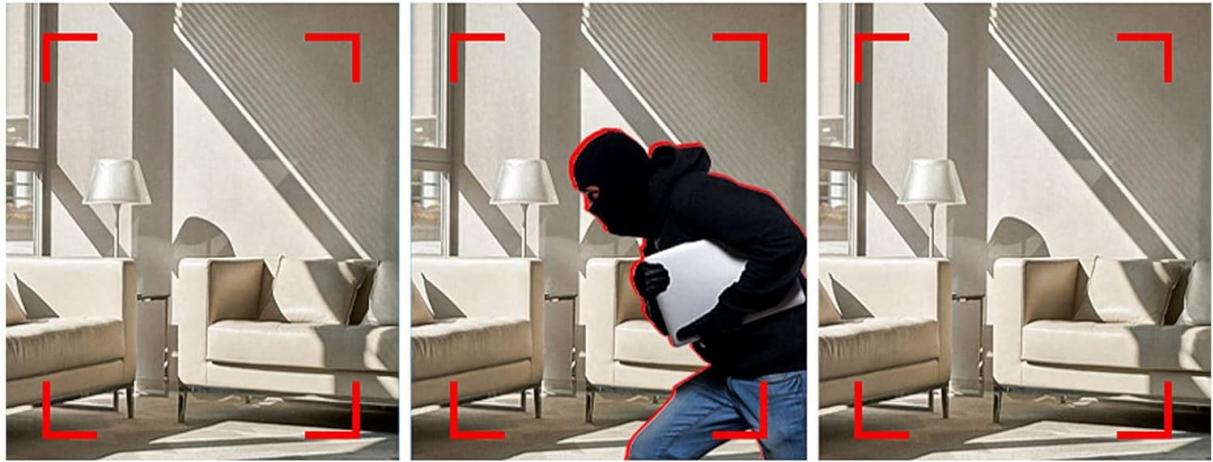
Figure 4.2: Example of PIR video recording, showing how the camera detects and records when motion is present in its field of view.
