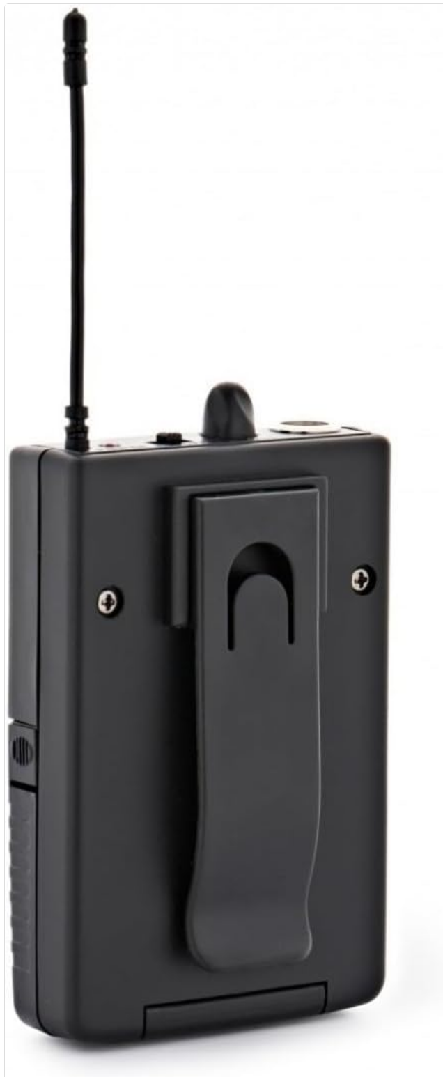
Figure 3.5: Rear view of the bodypack transmitter with belt clip.
