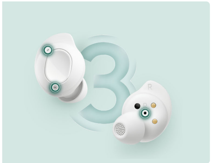
Image: Diagram showing the placement of three microphones on a Galaxy Buds FE earbud for enhanced call clarity.
