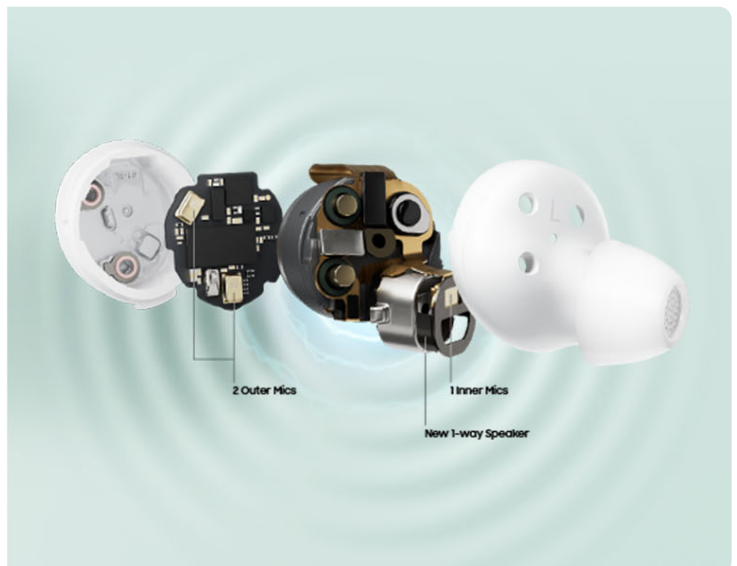
Image: Exploded view of a Galaxy Buds FE earbud, highlighting the 1-way speaker and internal microphone components.
