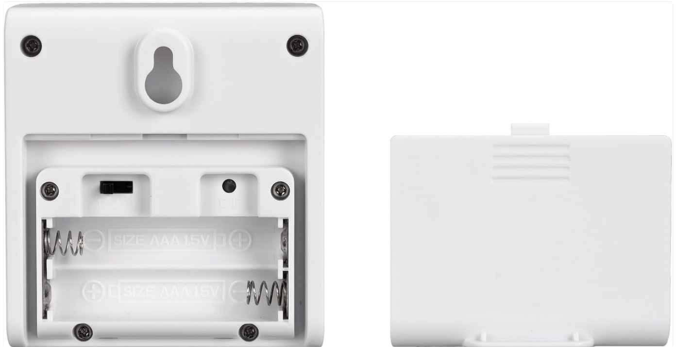
Figure 3: Rear view of the sensor, illustrating the battery compartment and the channel selection switch.
