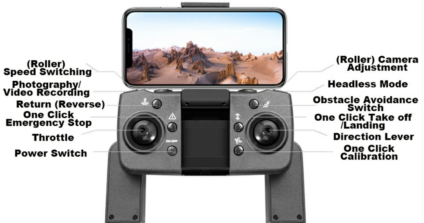
Image: Diagram illustrating the functions of the remote control, including speed switching, photography/video recording, return, emergency stop, throttle, power switch, camera adjustment, headless mode, obstacle avoidance switch, one-click takeoff/landing, direction lever, and one-click calibration.
