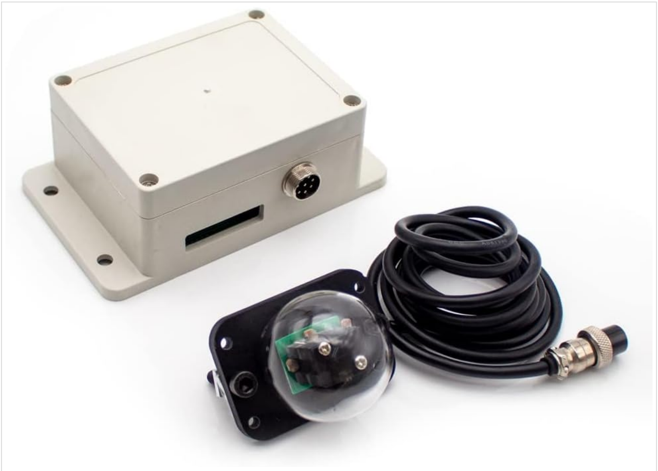
Figure 1: Main Controller, Light Sensor, and Cable
