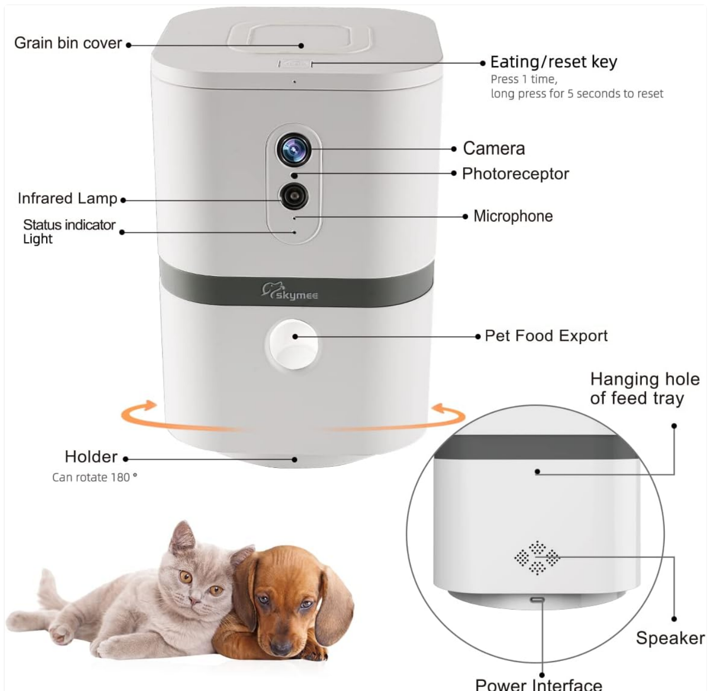
Image 2.2: Detailed diagram of the Petalk AI II components, including the grain bin cover, eating/reset key, camera, photoreceptor, microphone, infrared lamp, status indicator light, pet food export, hanging hole for feed tray, holder (rotates 180°), speaker, and power interface.
