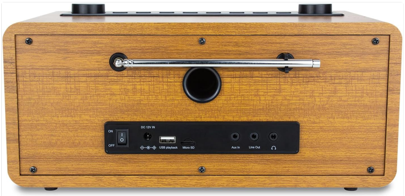
Figure 3.3: Rear view of the Ocean Digital WR-860, displaying the connection ports. From left to right, these include the ON/OFF power switch, DC 12V IN port, USB playback port, Micro SD card slot, Aux In port, and Line Out port. A telescopic antenna is also visible.
