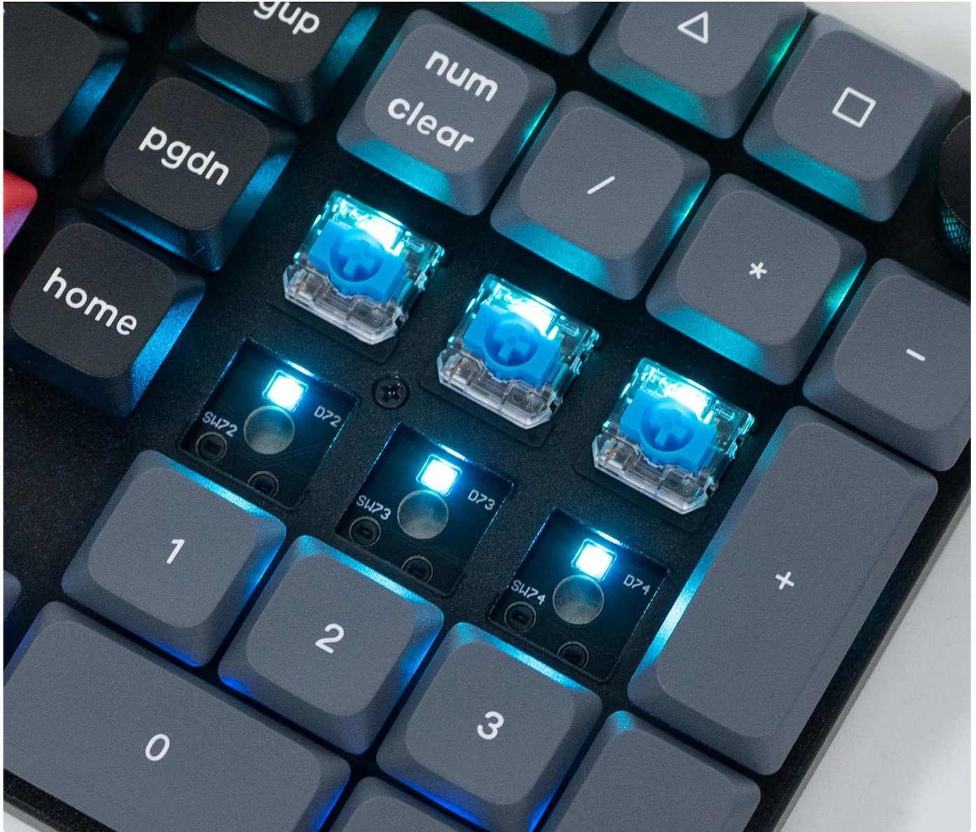
Image: Illustration of the hot-swappable feature, showing a low-profile Gateron switch being removed and double-shot PBT keycaps.
