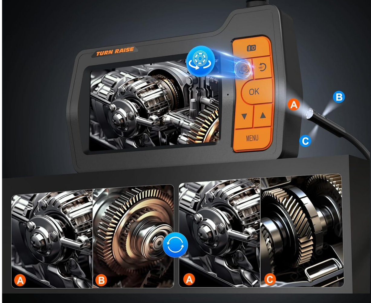
Image 4.3: The split-screen view feature, demonstrating how the monitor can display multiple camera feeds simultaneously for enhanced inspection in confined spaces.
