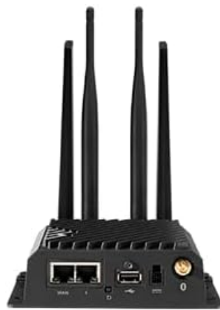
Figure 2: Rear view of the Cradlepoint R920 router, illustrating the various ports and antenna connectors. This includes Ethernet ports, USB port, and cellular antenna connections.
