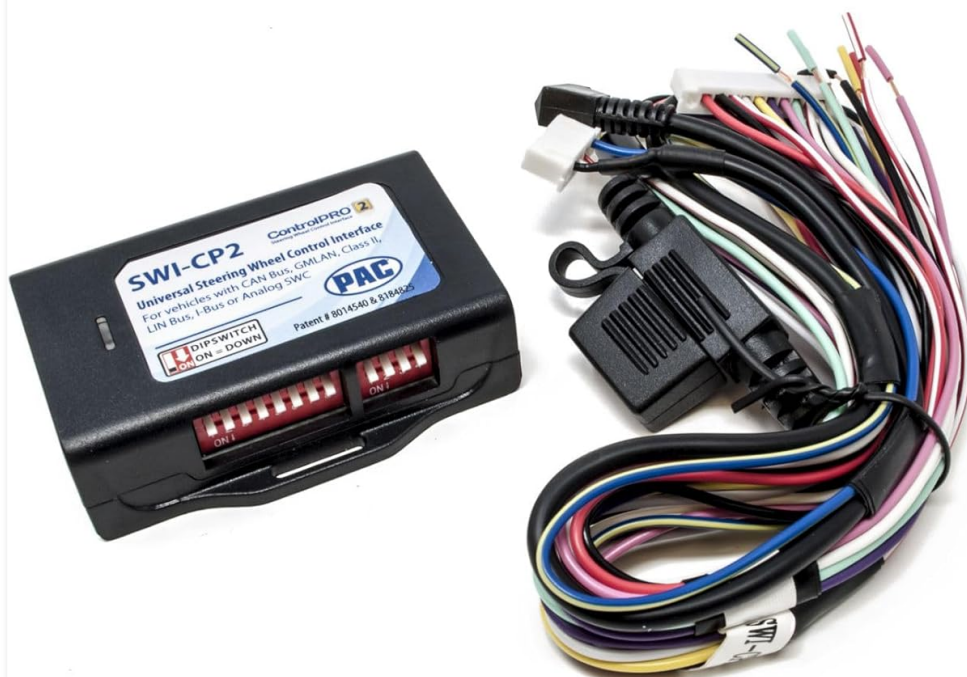
Image: The PAC Audio SWI-CP2 Universal Steering Wheel Control Interface and its accompanying wiring harness, essential for integrating steering wheel controls with the Alpine receiver.
