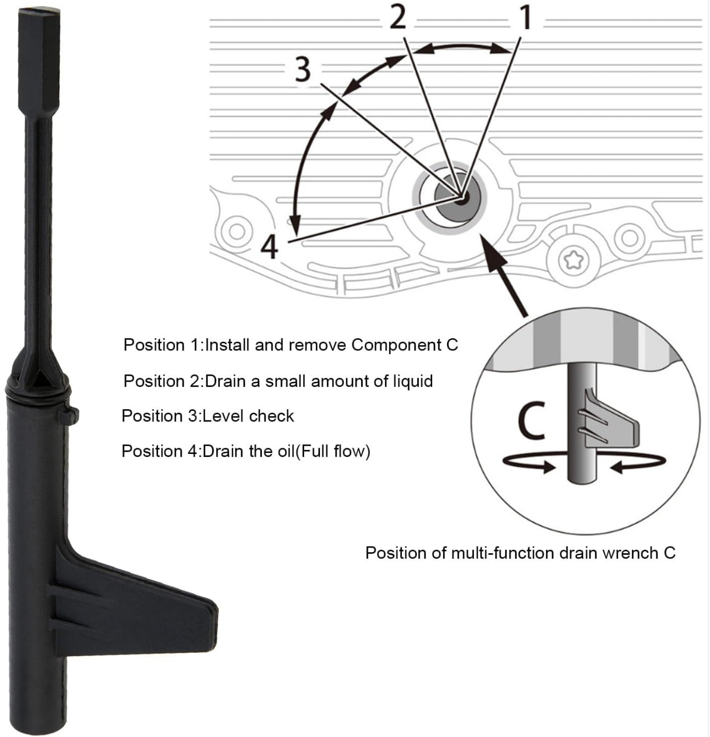
Figure 7: Diagram illustrating the four operational positions of the multi-function drain wrench (Component C).
