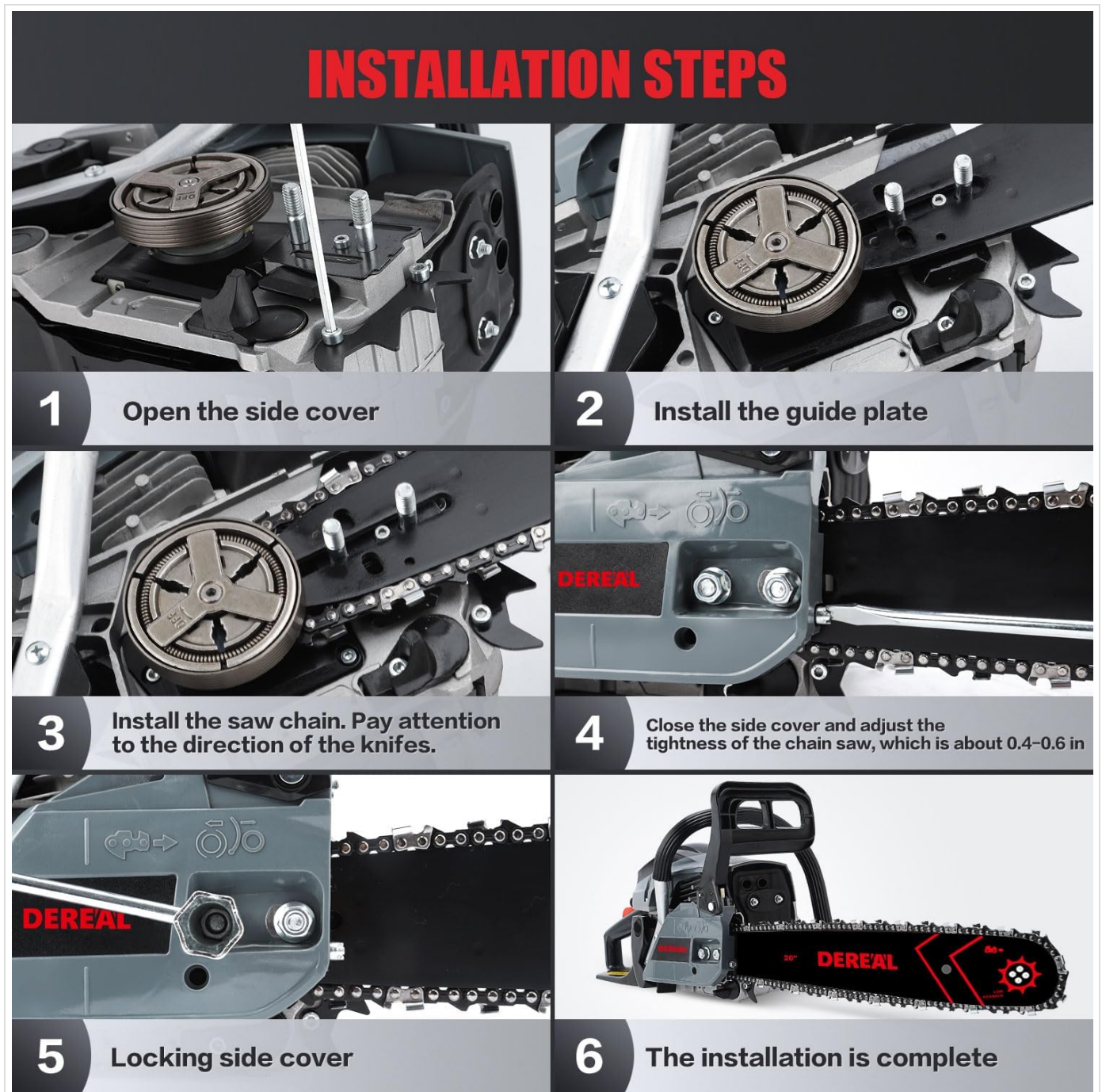
Figure 4: Step-by-step visual guide for chainsaw assembly. This image demonstrates how to open the side cover, install the guide plate, install the saw chain (noting direction), close the side cover and adjust chain tightness, secure the locking side cover, and shows the completed installation.
