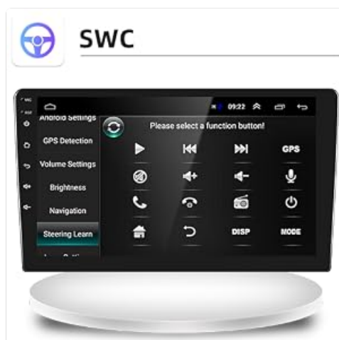
Image: The car stereo display showing the "Steering Learn" menu, where users can configure steering wheel control buttons.
