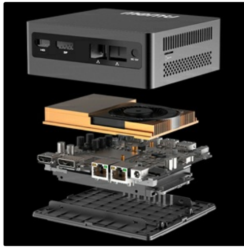
Image 4.1: An internal view of the Mini PC's cooling system, showing the fan and heat sink designed to dissipate heat and maintain stable performance.
