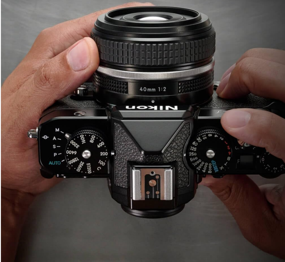
Figure 3.1: Top Dials for Manual Control
