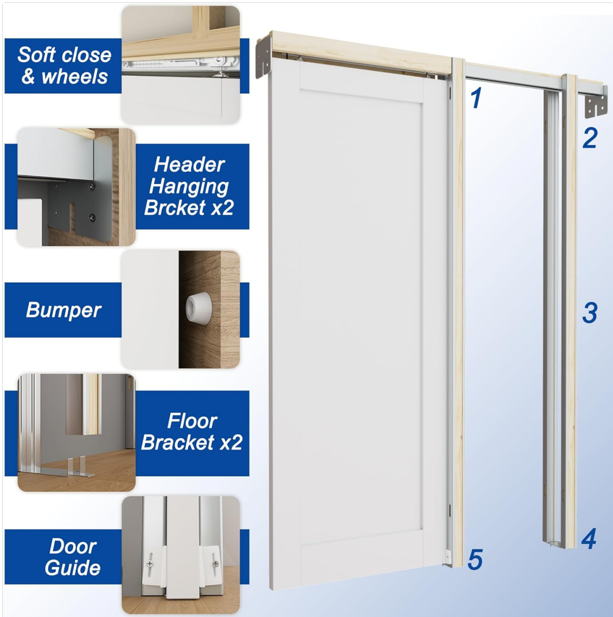
Image: Exploded view of the pocket door components, illustrating the soft-close mechanism, header hanging brackets, bumpers, floor brackets, and door guides.
