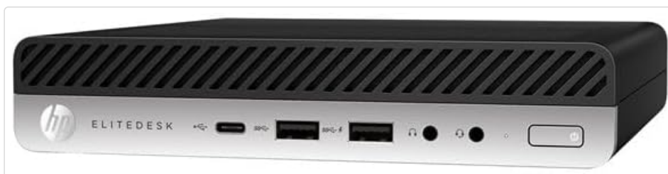
Figure 3.2: Front view of the HP EliteDesk 800 G5 Mini PC, showing the headphone jack, USB-A 3.1 Gen 1 (charging), USB-A 3.1 Gen 2, USB 3.1 Type-C Gen 2, and power button.
