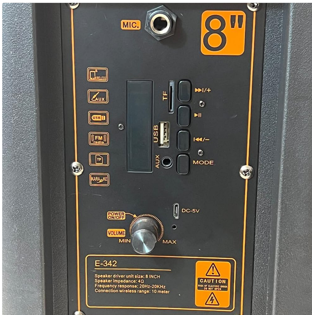
Image: Close-up view of the speaker's control panel, showing the microphone input, USB and TF card slots, AUX input, mode button, volume knob, and DC-5V charging port.
