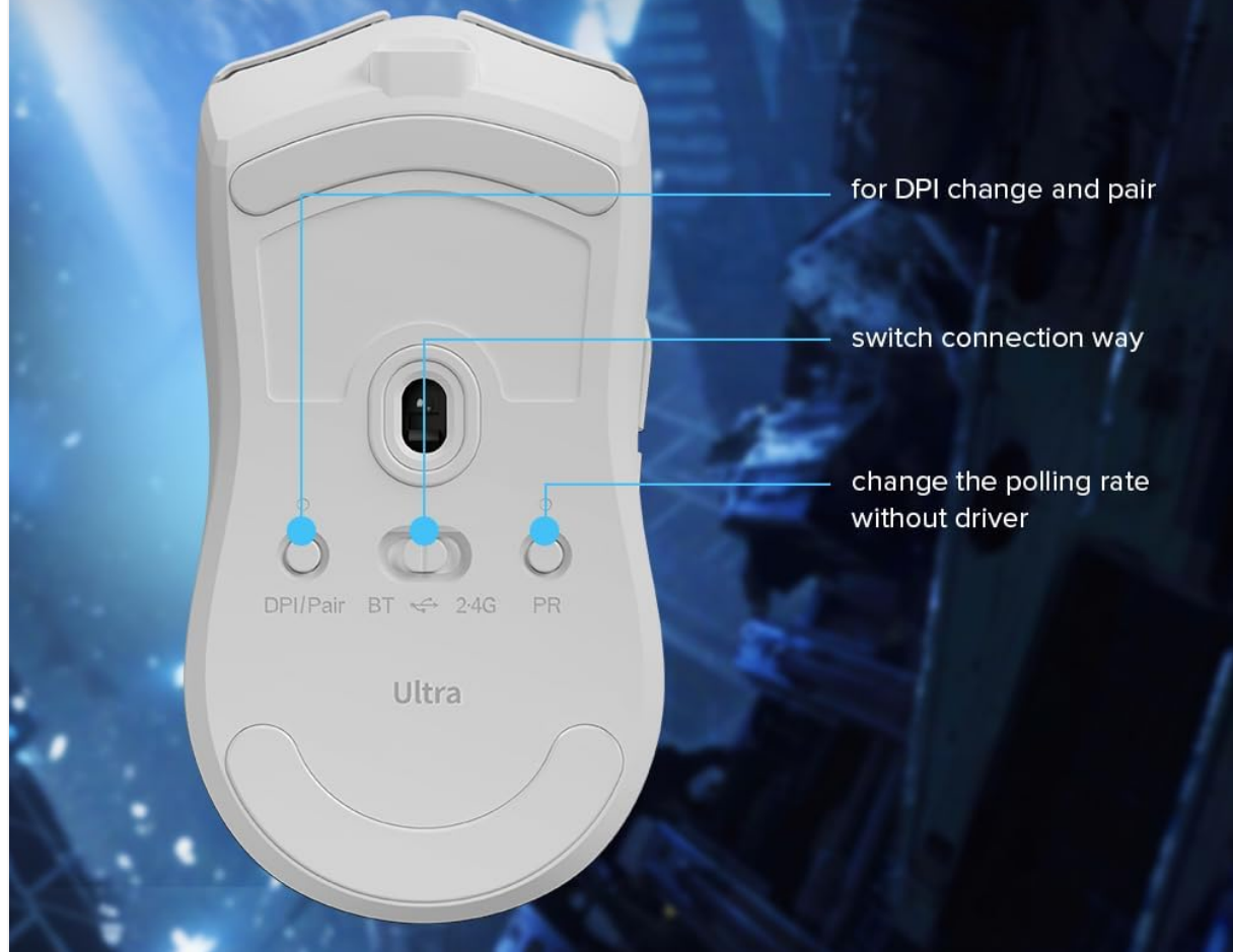
Figure 3: Bottom button layout for DPI, Polling Rate, and Connection Mode
