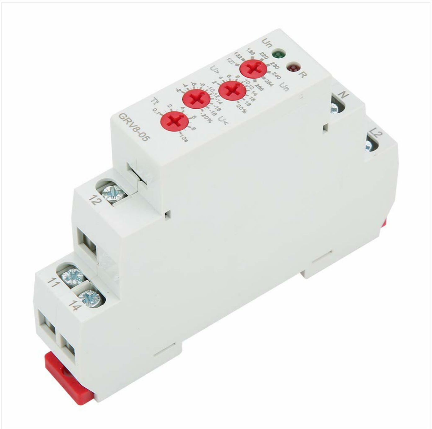
Figure 6.1: Close-up view of the adjustment knobs for rated voltage ( U_n ), overvoltage ( U_{>} ), undervoltage ( U_{<} ), voltage unbalance ( U\% ), and action delay time ( T_t ).
