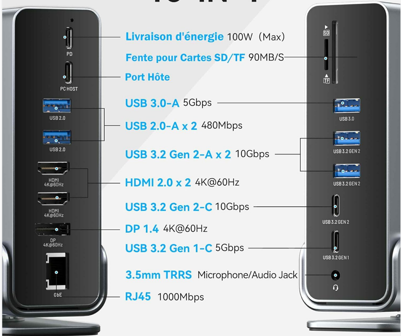
Image: Detailed diagram illustrating all 16 ports on the VENTION docking station, including their types and maximum speeds/resolutions.
