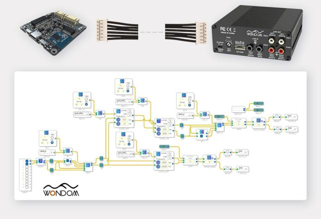
**Figure 4: SigmaStudio Programming Setup.** This image illustrates the connection between the DSP unit and an ICP5 programmer, along with a visual representation of the SigmaStudio graphical programming interface.
