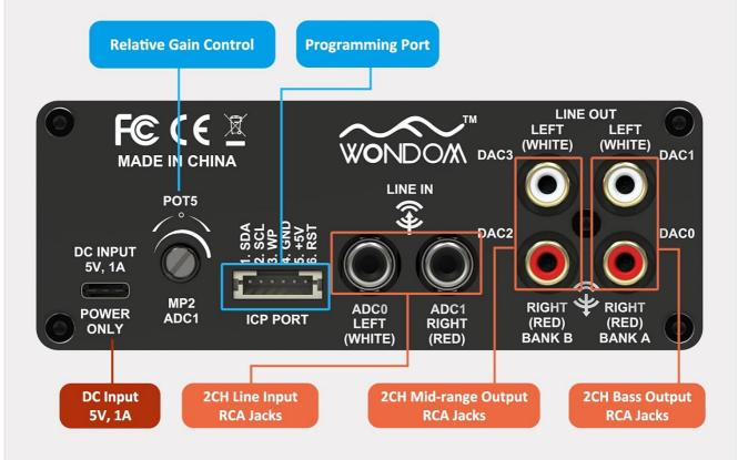
Figure 1: Rear Panel Connections. This image shows the rear panel of the ADAU1701 DSP Preamp, highlighting the DC Input (5V, 1A), ICP Port, Line In (ADC0 Left, ADC1 Right), and Line Out (DAC0 Right, DAC1 Left, DAC2 Right, DAC3 Left) RCA jacks.
